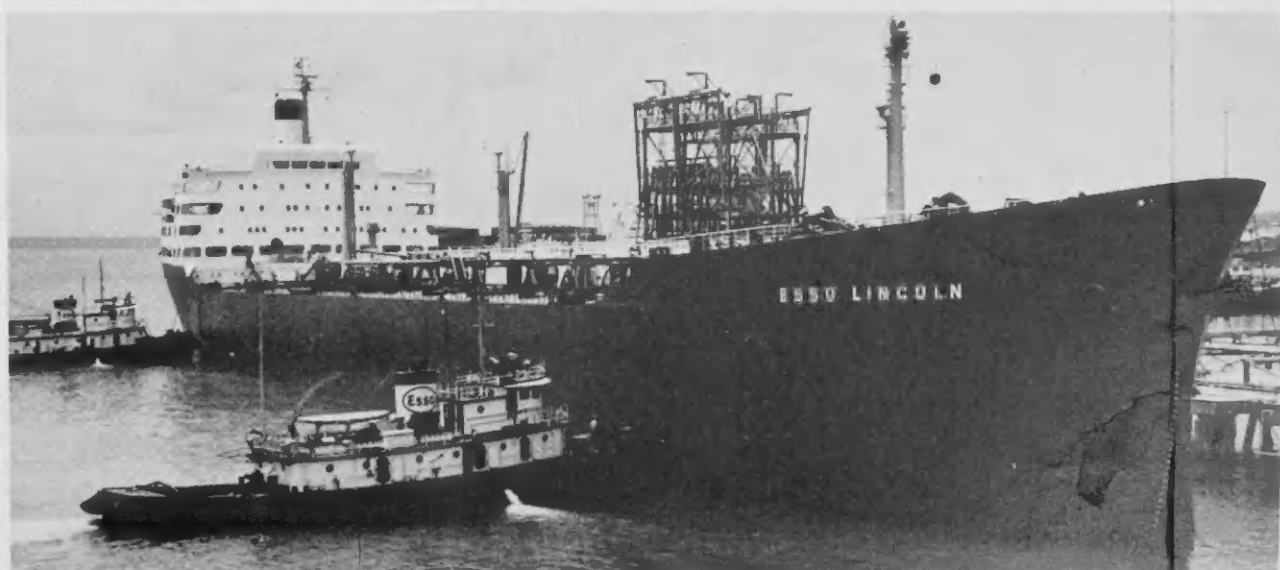
THE ESO LINCOLN moved into San Nicolas Harbor Sept. 22 on the first leg of its maiden voyage. The new tanker was launched in December, 1961, the first of four sister ships built with all accommodations aft.
